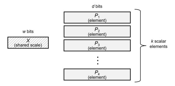
All k elements  $(P_i)$  have the same data type and, therefore, the same bit-width. The scale factor X is shared across all k elements. The data types of the elements and scale are chosen independently. In this sense, MX can be seen as a mechanism to build a vector data type from scalar data types.
