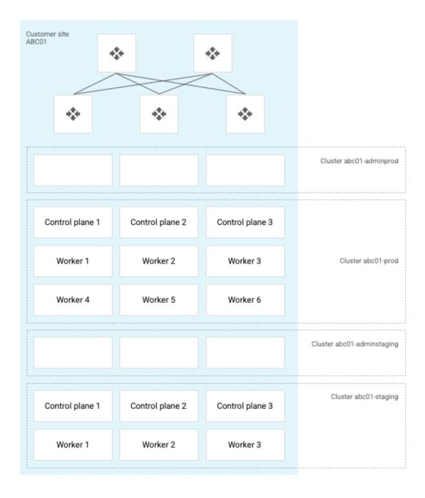
When VMware or other virtualization is used, the ESXi hosts or equivalent can be spread across several racks. This approach enables the VMs to be spread across hosts, as shown in the following diagram:
