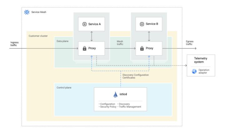
When using Service Mesh to secure service traffic within a cluster, you should also secure external traffic. Don't allow direct connections to clusters for management operations by users or automated processes. Instead, connect to clusters by using the private on-premises network or through the connect gateway.
